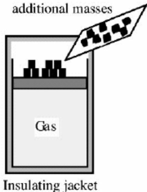
An ideal gas is contained in a cylinder with a tightly fitting piston. Several small masses are on the piston. (See diagram above.)
