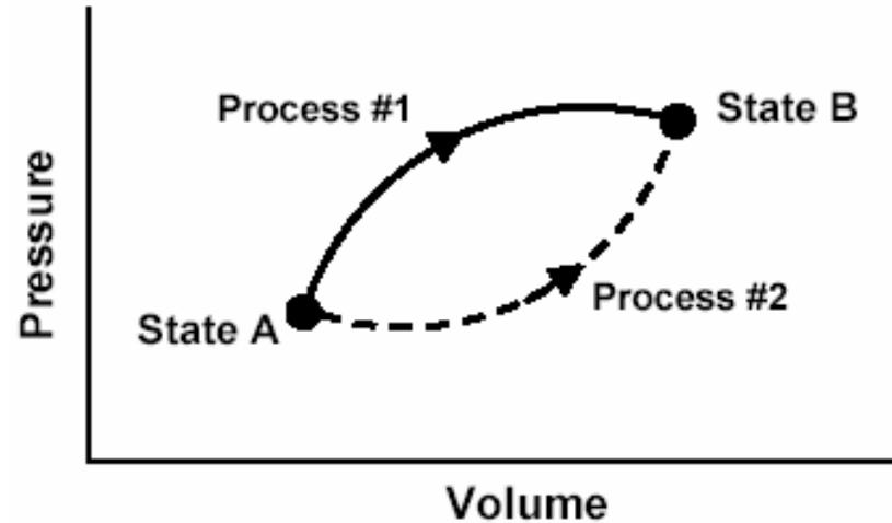
This  $P$ - $V$  diagram represents a system consisting of a fixed amount of ideal gas that undergoes two ***different*** processes in going from state A to state B:
