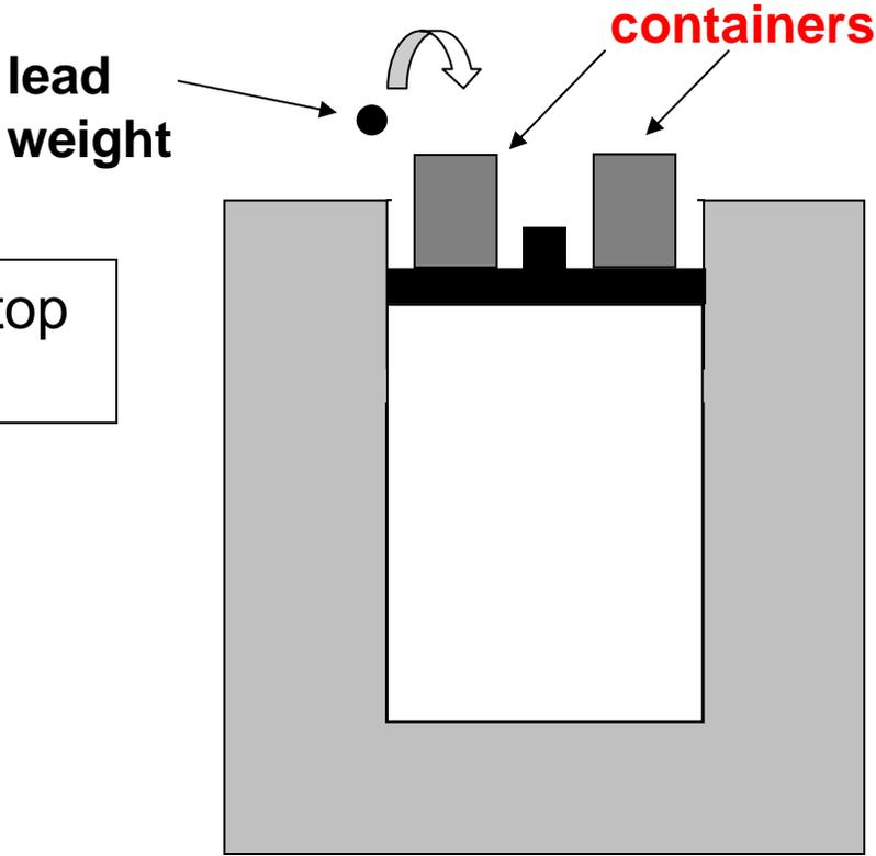
Small lead weights are gradually placed in the containers, one by one, and the piston is observed to move down slowly.
