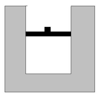
**Step 1.** We now begin Process #1: The water container is gradually heated, and the piston *very slowly* moves upward. At time *B* the heating of the water stops, and the piston stops moving when it is in the position shown in the diagram below:
