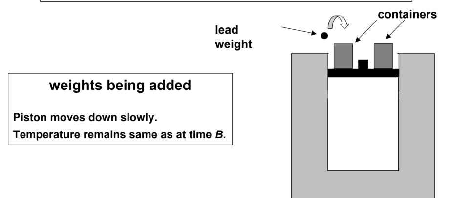
**Step 3.** At time *C* we stop adding lead weights to the container and the piston stops moving. (The weights that we have already added up until now are still in the containers.) The piston is now found to be at *exactly the same position it was at time* A.
