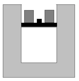
**Step 3.** At time *C* we stop adding lead weights to the container and the piston stops moving. (The weights that we have already added up until now are still in the containers.) The piston is now found to be at *exactly the same position it was at time* A.
