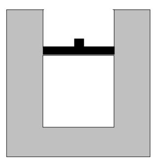
**Step 4.** Now, the piston is locked into place so it *cannot move*; the weights are removed from the piston. The system is left to sit in the room for many hours, and eventually the entire system cools back down to the same room temperature it had at time *A*. When this finally happens, it is time *D*.
