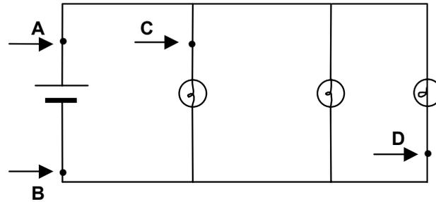
In this circuit, rank the *amount of current* flowing past the four points A, B, C and D.
