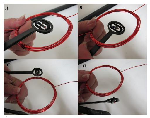
Hold the Magnaprobe at different locations to check the direction of the magnetic field when the coil is connected to the battery (see photos above). Which way does the needle point when you hold it: (A) above the center of the coil; (B) below the center; (C) near one side; (D) near the other side? Where is the north pole of the coil? The south pole? How do your answers change when you reverse the connections to the battery terminals?
