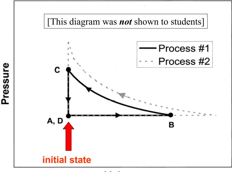
Beginning at time *A*, the water container is gradually heated, and the piston *very slowly* moves upward.
